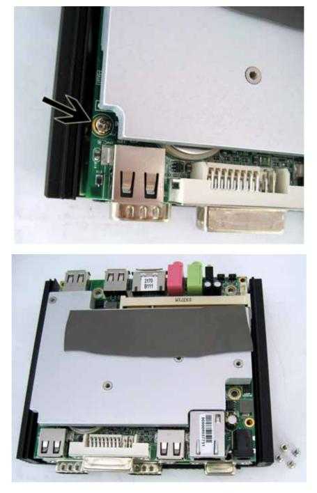
Hold the enclosure with one hand and remove the mainboard with you other hand upwards. (ATTENTION: straight upwards, not slant, because you will maybe damage the pins.)
