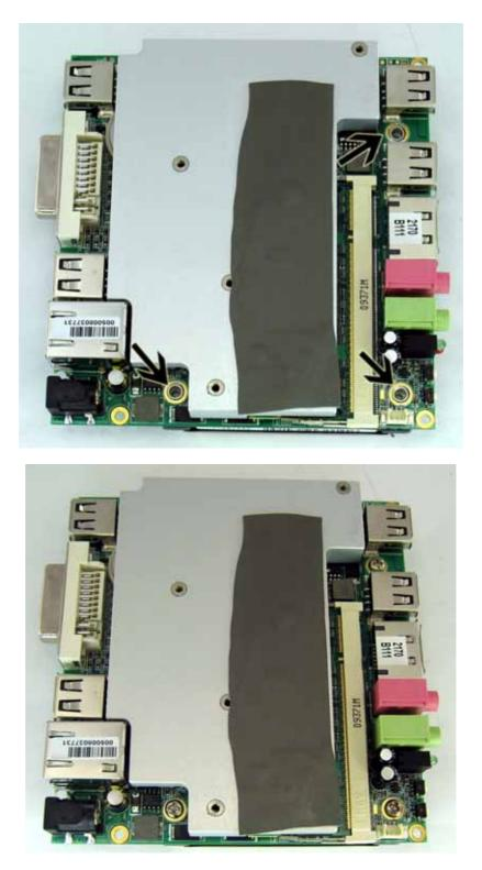
Now, you can bring up again the mainboard. Please be careful, you should not damage the pins. If the mainboard is set on the right position, press it down, till you not see the pins any longer. Now the mainboard can be screwed.
