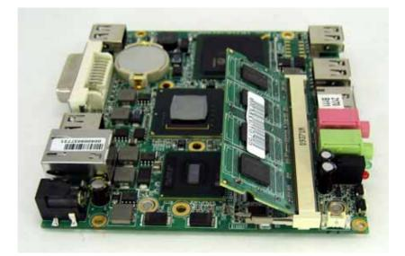
Place the RAM to the slot in push it down till the RAM is engaged. After that, bring the cooling unit back on the System and fix it.
