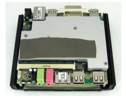
Set up the Cover of the enclosure back on the top (there is only on possible way), bring the slot plate back on the right position and fix all of the screws.
