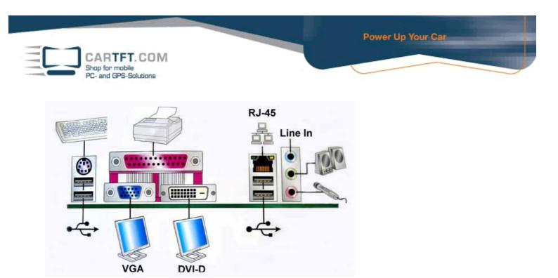
On the I/O panel you will find the following connections: DVI output, VGA, four USB 2.0 ports, one GigaLAN bush as well as the standard audio ports.
