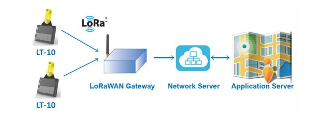
Before starting communication LoRaWAN<sup>TM</sup> gateway and LT-10 LoRa<sup>®</sup> trackers, please refer to LoRaWAN<sup>TM</sup> gateway's user manual to set the LoRa<sup>®</sup> settings by GlobalSat Configuration App.
