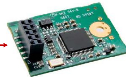
Optional: Attach USB Flash Disk Module (up to 8GB available) e.g. www.stec-inc.com
