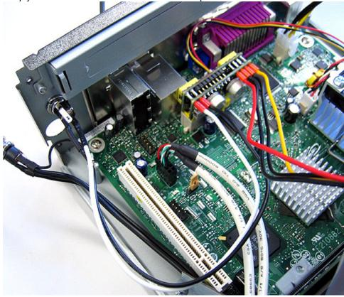
Otherwise the picoPSU120 gets connected with the adapter cables as described above.
