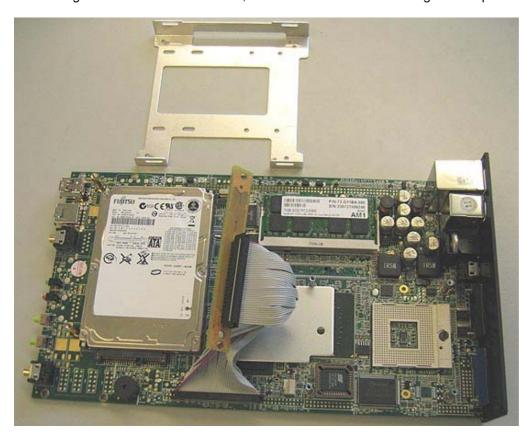
Then you take the CPU and check the arrangement of the pins, so that the CPU sinks into the socket without any reluctance and effort. After that you close the lock of the socket with a slit screwdriver.
