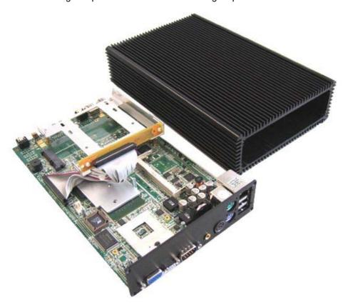
Now the motherboard is lying in front of us and we can begin with the installation of the SO-DDR2 RAM:
