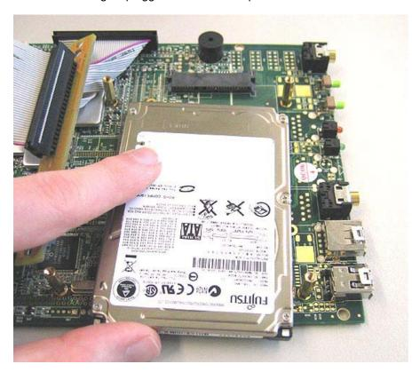
On the rear of the motherboard you can fasten the SATA HDD with 4 screws:
