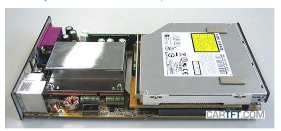
Before the motherboard gets slid in the case again, the fake-drive blend has to be removed of the case, so that the correct CD/DVD-ROM can be used.
